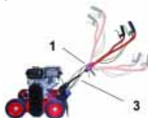
Fig. 9 - model 519-50 Scarifying depth / 519-50: Turn the key "8" until it engages. Then proceed as for model 519.
