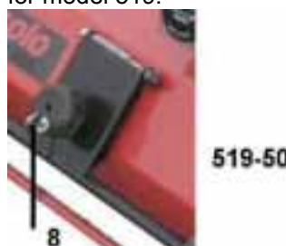
Fig. 9 - model 519-50 Scarifying depth / 519-50: Turn the key "8" until it engages. Then proceed as for model 519.
