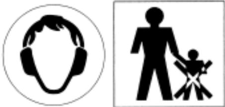
Earmuffs must be worn. Do not allow children near the machine when in operation.
