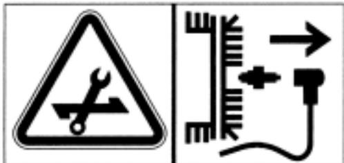
Warning. Always disconnect the cable from the engine spark plug.
