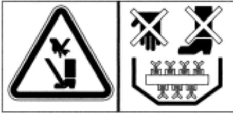
Danger of injury to both upper and lower limbs. Do not put hands or feet inside the cutting element while in motion.
